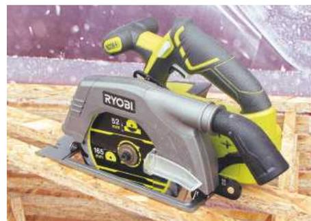
Use this one on sheet material and constructional timber
